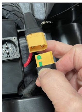
Figure S: Disconnect battery.
