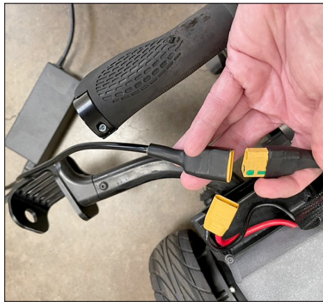
Figure P: Battery connected to charger.
